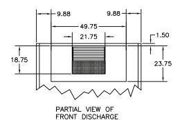
NOTES: 1. Dimensions in inches. 2. All units are rear return airflow configuration. 3. Recommended minimum service clearances are as follows: a. Front and rear — 30 in. (762 mm) b. Left or right side — 65 in. (1651 mm) for coil removal c. Side opposite coil removal — 20 in. (508 mm) Fig. 5 -
